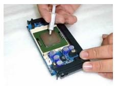
Applying thermal compound to the processor.
